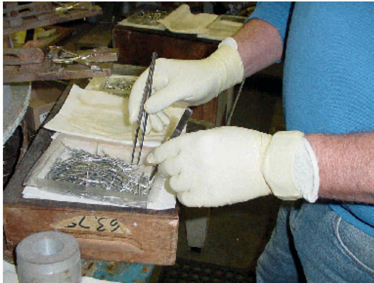
Figure 1 Worker is exposed to health and safety risks of acid flux, solder/flux fumes, residue and proximity to heating flame.
