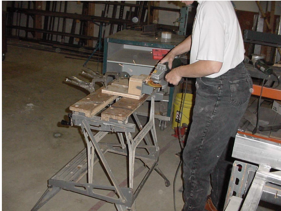
Clamping device is in a fixed location creating awkward postures
