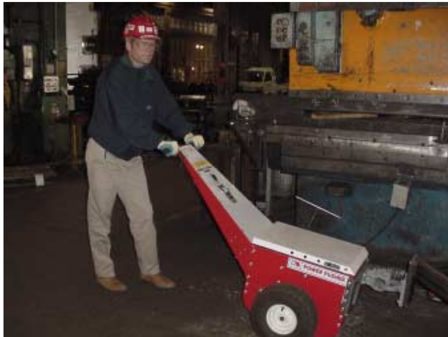
Power Pusher operates with hand controls to move the dollie and scissors lift
