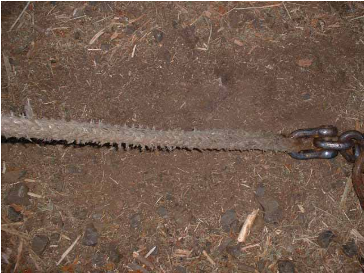
Figure R6. Rope appearance. Fuzzed filaments and tufts (local accumulation of fuzzed filaments) on the end of a skidder winch line. Continuous abrasion by the ring sliders created this condition. Rope failures have occurred near the buried tail of this eye splice, but not in the splice section itself. This is considered an acceptable wear condition for this application as the skidder winch line. Synthetic winch lines which experience cut strands that are not taken out of service or repaired (spliced) should be used with appropriate clearance from the probable failure zone. OR-OSHA 437-007-0605 exempts skidder winch lines from the out of service requirement because of expected failure and operator protection.
