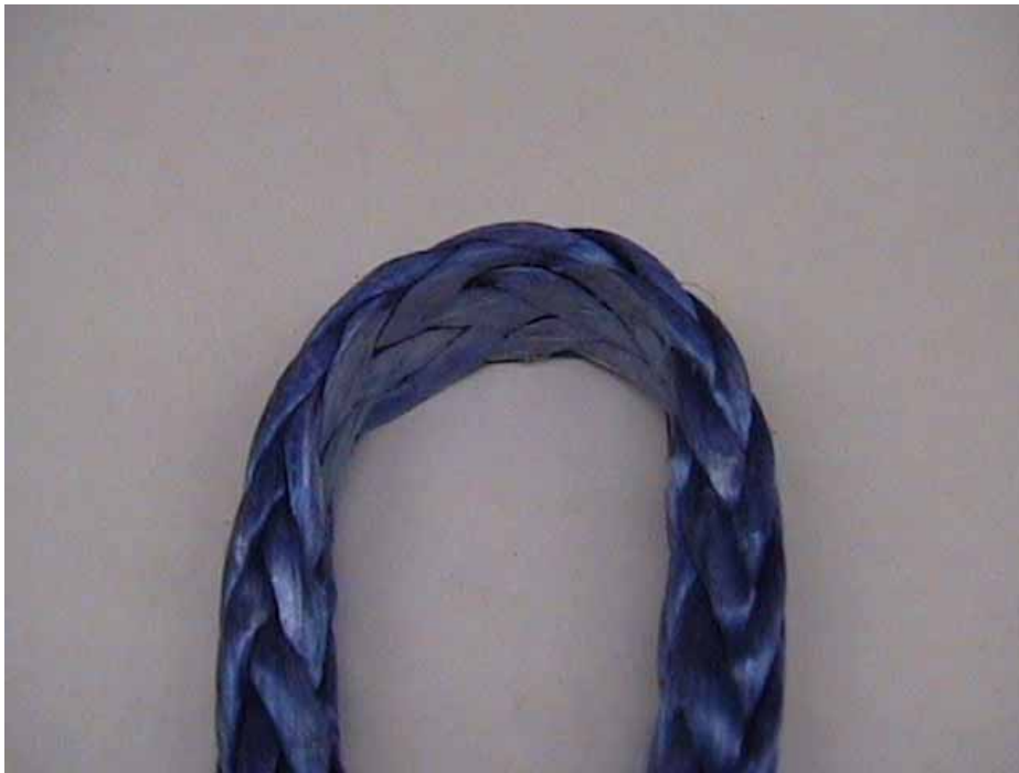
Figure R12. Fiber set due to compressive loading around the barrel of a drum winch. Note slightly glazed appearance. Flexing of the rope should eliminate this appearance and allow for continued use of the rope.
