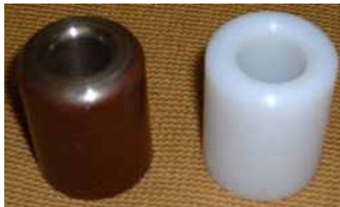
Figure 11. B-5 Steel nubbin and UHMW-PE nubbin
