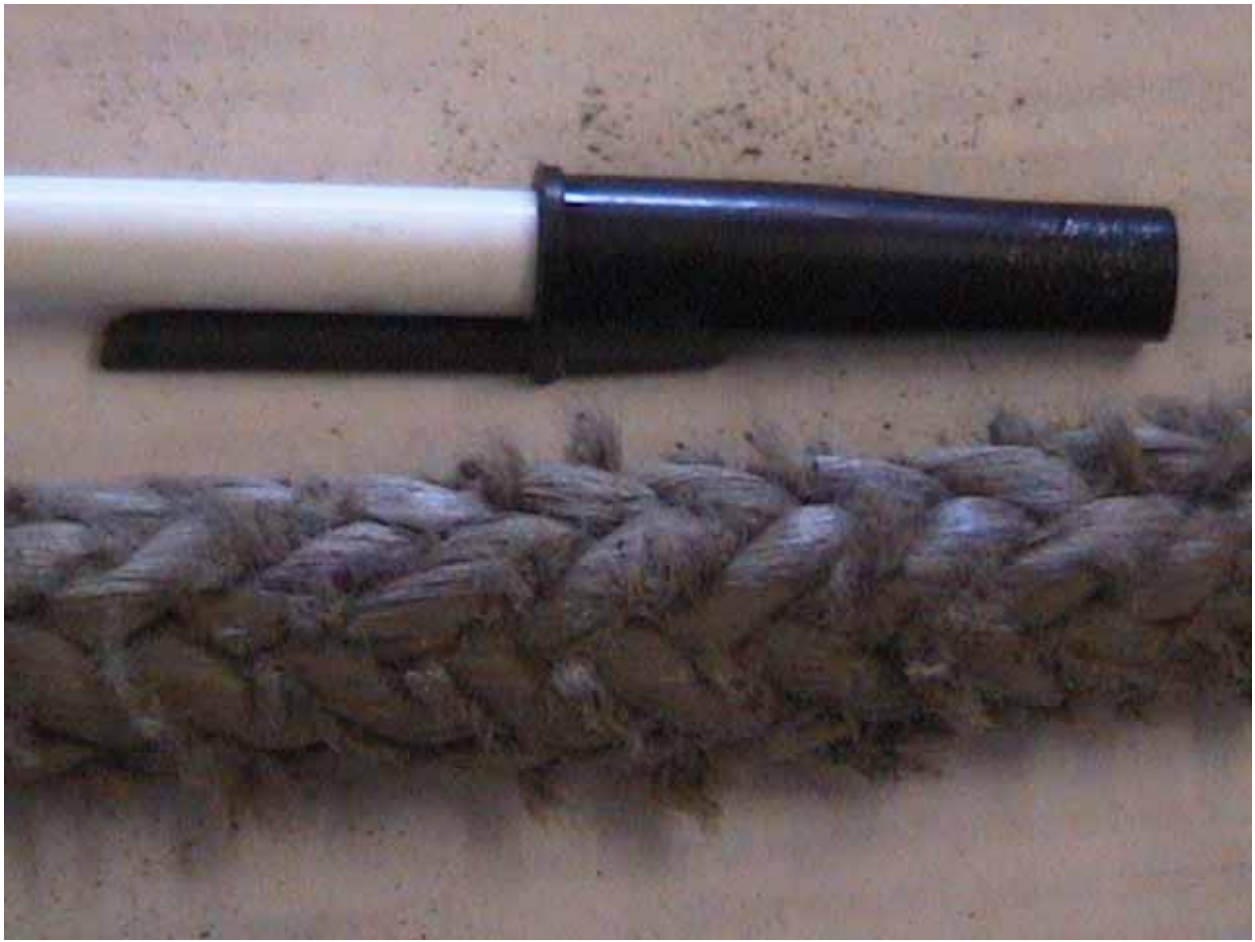
Figure R8. Section of a 3/8-inch ASB synthetic rope wrapper with accumulation of cut filaments.
