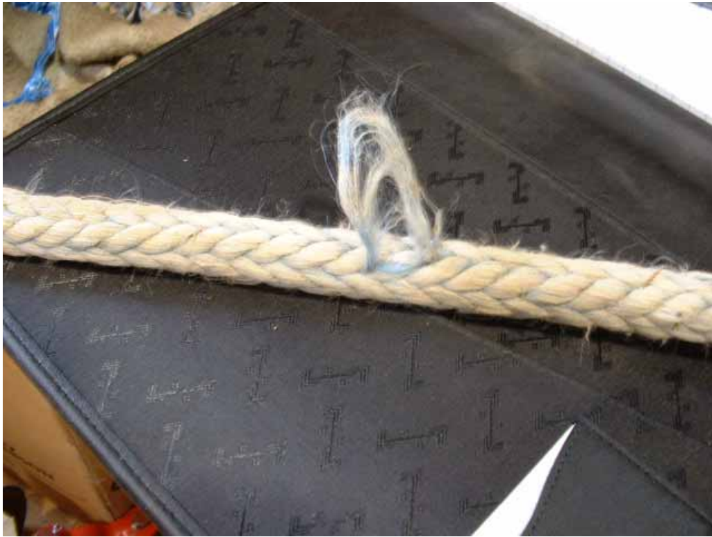
Figure R11. Pulled yarn (collection of filaments) from a single strand of a 12 strand ASB synthetic rope. Pulled yarns and strands should be re-threaded to prevent snagging and further malformation of the rope structure during operation.
