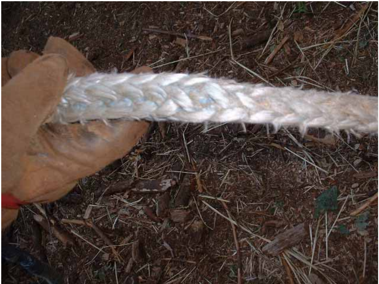
Figure R7. Section of skidder winch line from Figure R6 located away from the working end. Note reduction in quantity and quality of tufts. Also note residual blue coating on the internal portion of the strands.
