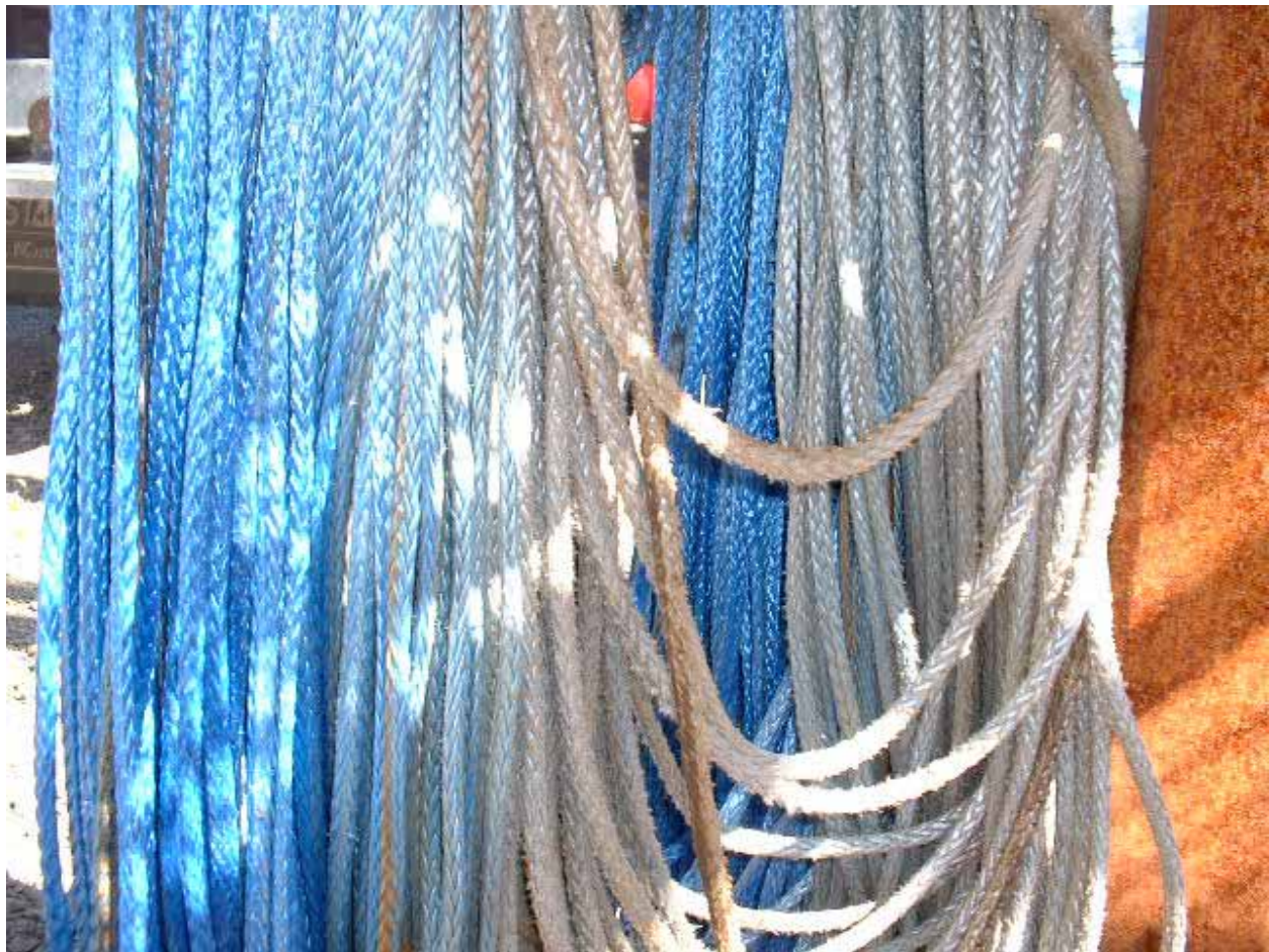
Figure R5. Gradation of color with normal use. Shown is the 3/8-inch ASB synthetic rope mainline for a Koller K300 yarder.
